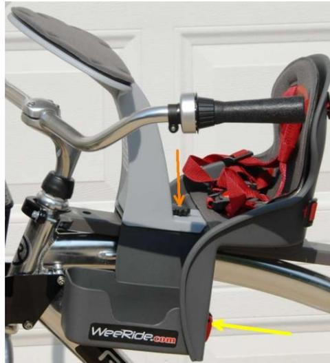
Once installed, the height of the child's foot rests could be individually adjusted utilizing a clever cam-lock (**yellow** arrow above) without having to resort to tools. In all, the assembly and installation of the unit required less than 15 minutes.
